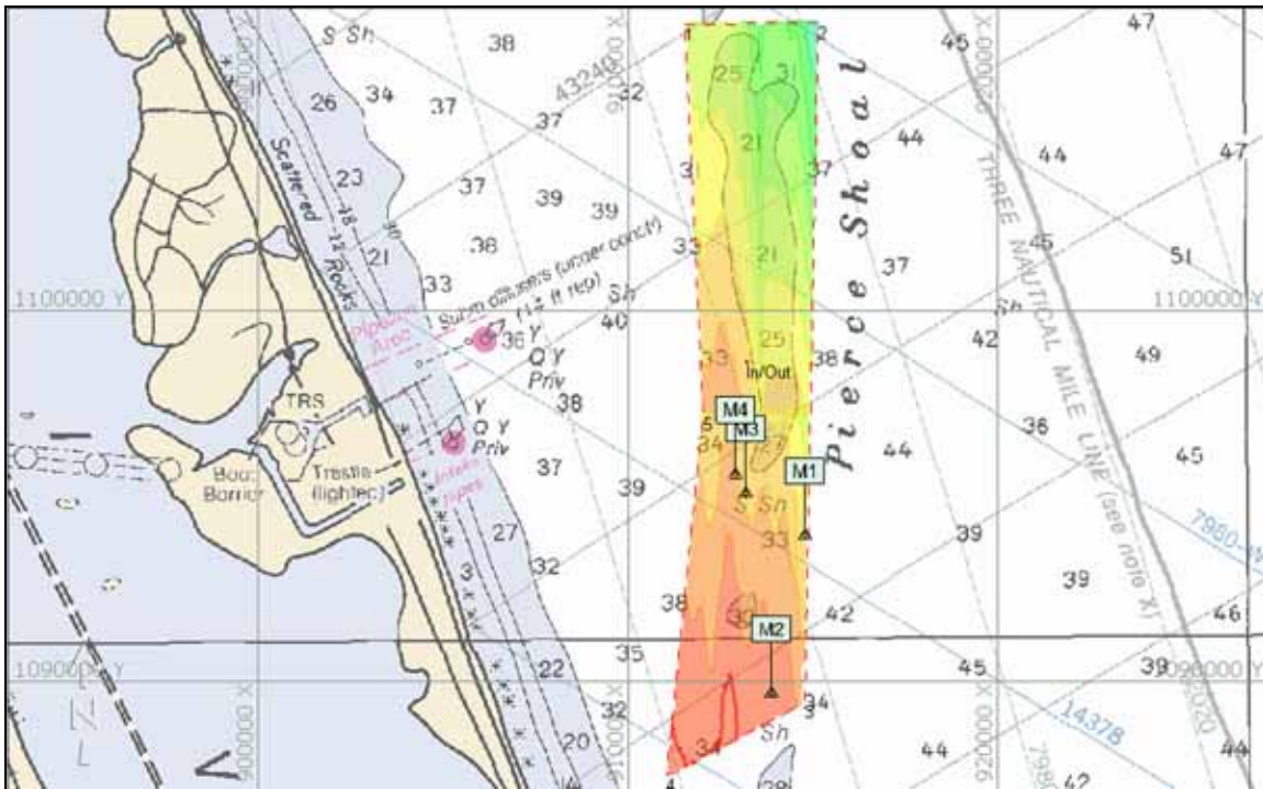
Figure 20. Magnetic anomalies, labeled in white, located within Borrow Area D. (NOAA Raster Chart No. 11474 “Bethel Shoal to Jupiter Inlet”).
